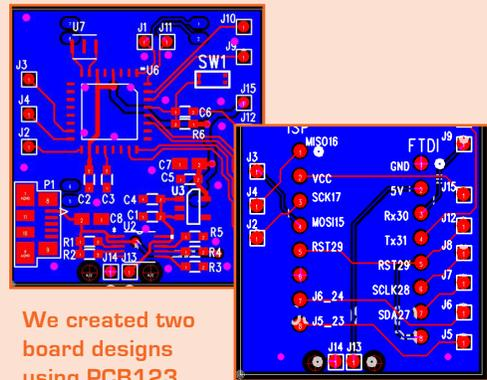
We created two board designs using PCB123, one for the watch itself and the second for the test/bootload station needed to program the watch.
