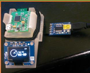
Concurrent with the jig design, the mechanical team got started on a watch enclosure and test/programming jig that would provide incoming QA and deploy the Arduino bootloader.
