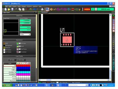
tip information. Reference designators automatically are synchronized; as the schematic's electrical network is further developed, "rat's nest" connections appear in the layout, ready to lead the user through the place-and-route process. It is worthwhile to note that, in this specific example, the information has been reviewed and certified as correct by NXP; the user can use this part with confidence that the landing pads
